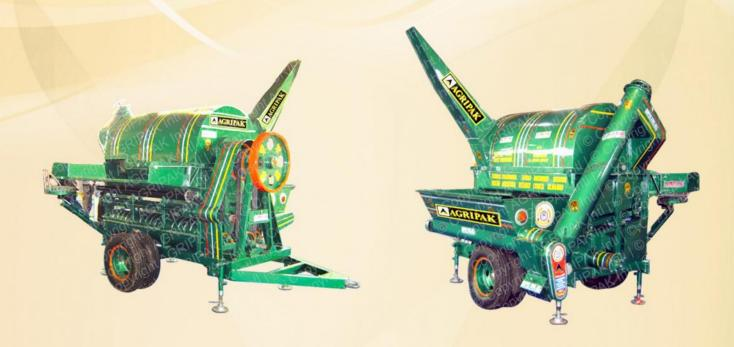
AGRIPAK PADDY/RICE THRESHER is a Tractor PTO Driven and can be used with separate Diesel Engine. Best alternate for those who are operating manually. Operation of this Thresher is depend upon the Axial Flow system.
